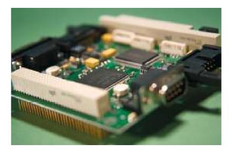
Compact and self-stacking, Kvaser PC104+ complies with the fexible PC/104 Plus specification. It represents a dual channel CAN Interface with a powerful microcontroller onboard.
